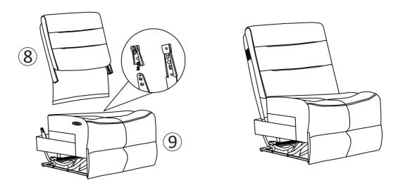
STEP 5: Install the corner position back 10 and 11 onto the corner seat 12.
