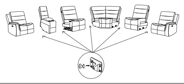
STEP 10: Connecting the power supply.
